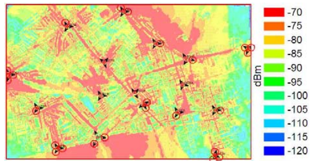
Fig. 5. Atoll predictions and antenna locations for the London scenario used in all simulations. Circled antennas were excluded from results collection.
